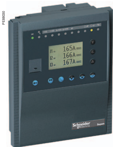
Sepam base unit (series 20 or series 40) with integrated advanced UMI.
